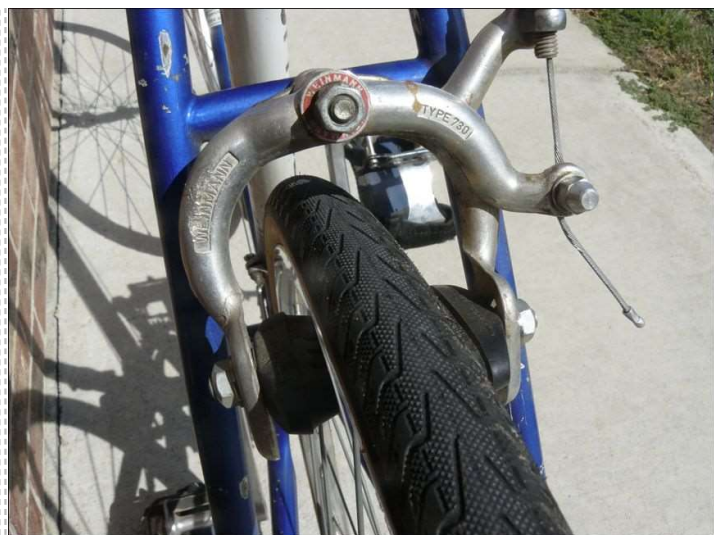
1972 Bottecchia Weinmann Side Pull Brakes
