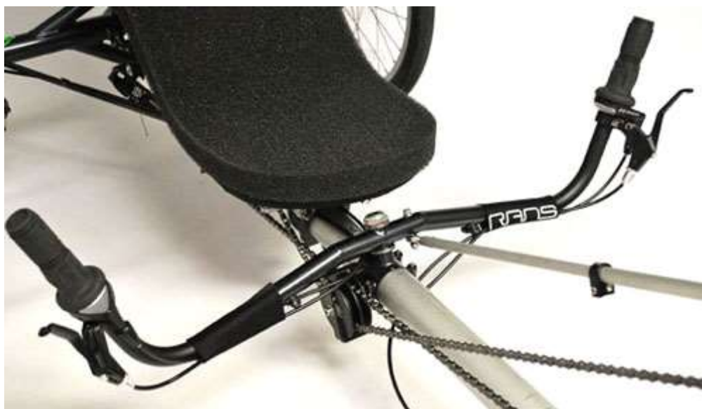
Topside bar install gull wing down
