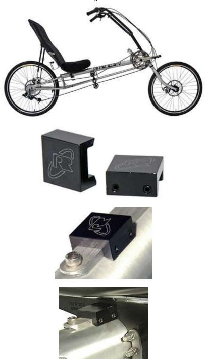
The <u>memory loc</u> marks where seat setting is, handy for when removed. It also prevents slippage. There is one slight drawback. You will lose 1 inch of aft seat adjustment, but if you are that close you could be against the stop anyway.
