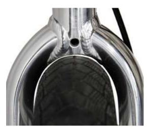
All wheel sets require disc brakes. Because of an adaptation of a frame, there is crank arm contact if rim brakes are mounted. With rim brakes and 650's in a tight turn while cranking will cause contact. There may be a long reach road brake that will work, none to date though.
