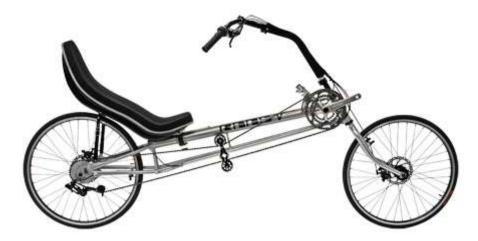
The fast version is set up with 26"x 20mm tires, T-Bar, and the M-5 seat, for a seriously fast ride.
