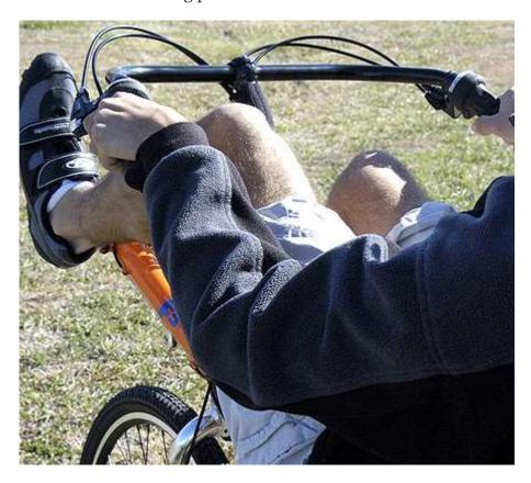
With the riser trimmed down 3" it keeps the bars out of view. Note: this may work for those in the 5'9" range and under.
