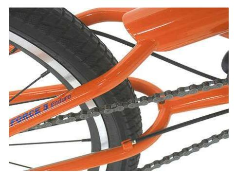
A slight twist to the frame design over the original F-5 allows big tire clearance, try a pair of 26x 2.3"s!
