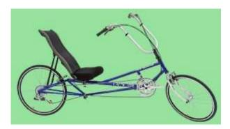
Using a custom fork and pushing the geometry the dual 26" Stratus XP is fairly compact, only 3" longer overall than the standard Stratus.
