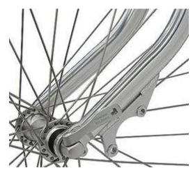
A custom fork with both canti and disc mounts is integral to making the Dual 26 Stratus XP a success.
