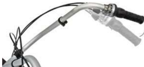
Adjust wrist feel by rotating grip tubes
