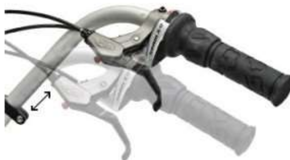
Adjust reach another way by moving the grip tube in or out.
