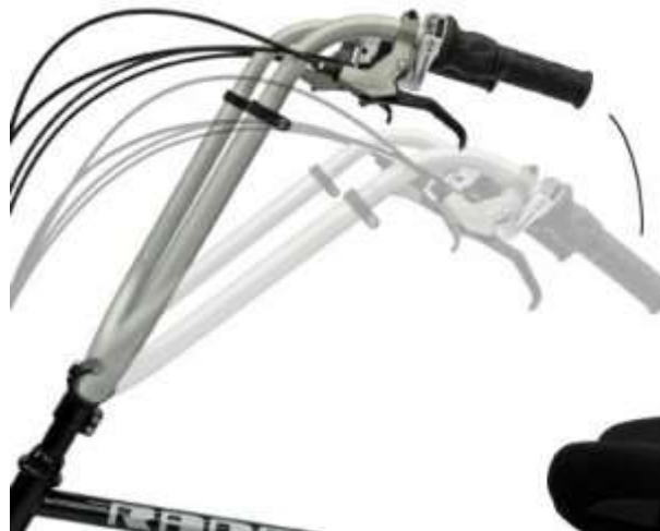
Tiller and reach change with rotation at the stem
