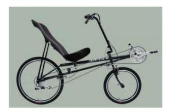
A longer wheelbase than other short wheelbase bikes of the time made the moving seat concept work.
