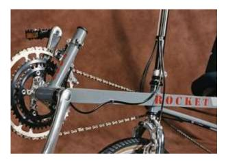
A MIG welded frame and square tube allowed the first Rockets to be mass- produced at our plant in Hays at a very reasonable price.
