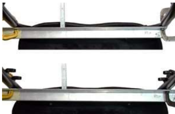
Top: two piece frame. Bottom: one-piece frame not modified.
