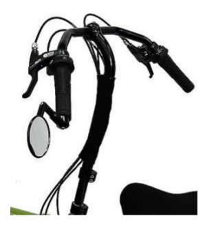
Set the tilt on your flip-it so it is more upright. Be careful not get the riser too far forward; it will make the bike overly sensitive in steering. The idea is to allow your arms to extend a bit, approximately 6" to 8". This opens up the cockpit and aids in mounting and dismounting. It has a neat feel to the handling we think you may like. With the bars forward and just clearing the knees you will have no worries about knees hitting the bars.
