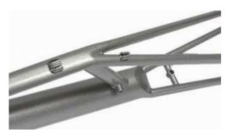
The load paths are direct allowing thinner wall tubes. Intersecting the main tube with oval seat stays makes for a better load transfer into the wall of the main tube. Again thinner walled tubes work here. The slant cut end on the main tube aligns the loads into the oval strut that completes the triangulation of the frames rear.
