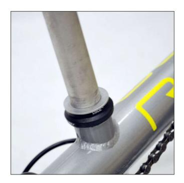
3. 1" steerer tubes need a steel sleave. Line up slots and keep steel sleeve at the top of the adjuster sleeve.
