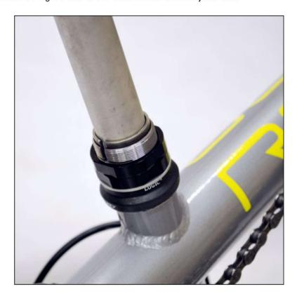
**5**. Now slide clamp over exposed threaded area and tighten clamp after there are no gaps or looseness in headset. (Do not use the consumer jamb nuts to make headset adjustment).
