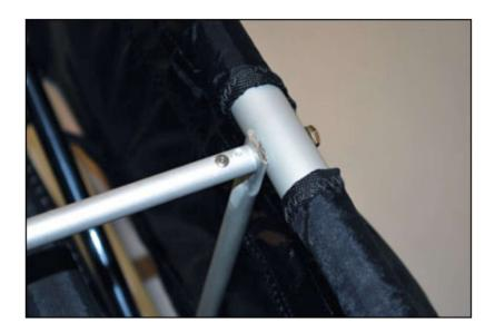
16. Take the 4 remaining 1/4" bolts, place a thin washer under the head, and apply lock tight. Use these bolts to install the aft and forward crossing tube (only the forward tube is marked) Install the cross tubes with the snap buttons facing forward.
