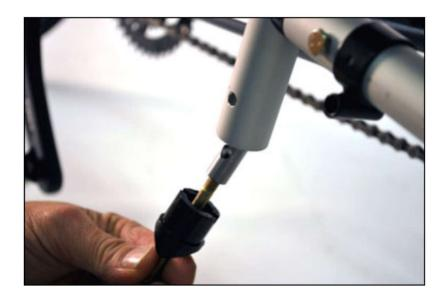
9. Of the 4 TC-1's (plastic saddles that insert into the ends of the tubes) two of them are cut off short, to create bolt clearance. Slip these into the bottom ends of the front of the side frames, and hold them in place with a small piece of tape.
