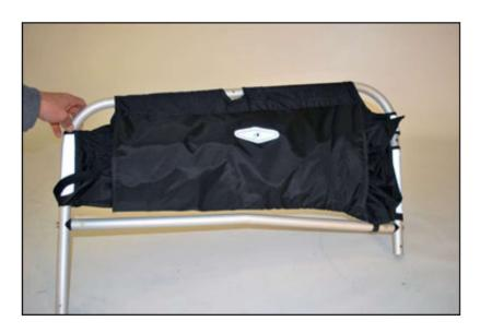
6. The side frames are now ready to assemble to bike. To prepare bike for assembly, apply tight lock to side frame attach hard points on the bike.
