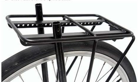
3. Attach the rack to the bottom dropouts using 5mm x12 bolt & (2) washers.
