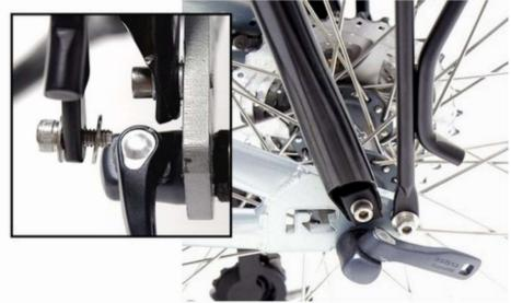
4. Slip clamp onto the sprint braces. Using the 5mm x25 bolt & (4) of the black washers, fasten to the corresponding holes on the rack. Tighten with the 5mm nut.
