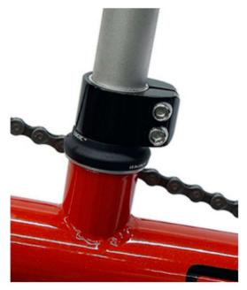
4. Slide riser w/ collar over stem tube & tighten at 1/8" above the lower collar. Do not tighten lower collar at this time.
