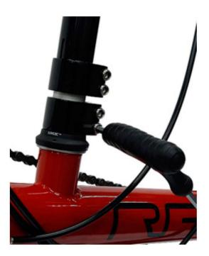
7. After lower collar is set, loosen top clamp & re-tighten riser height at best location for the rider.
