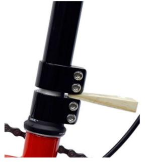
5. Line up bottom collar w/ wheel & tighten ightly.
