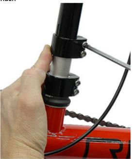
6. Remove play in headset by using a wedge to exert pressure between the collars. Insert wedge & tap lightly. Tighten lower collar when all play is gone & fork turns smooth & freely.
