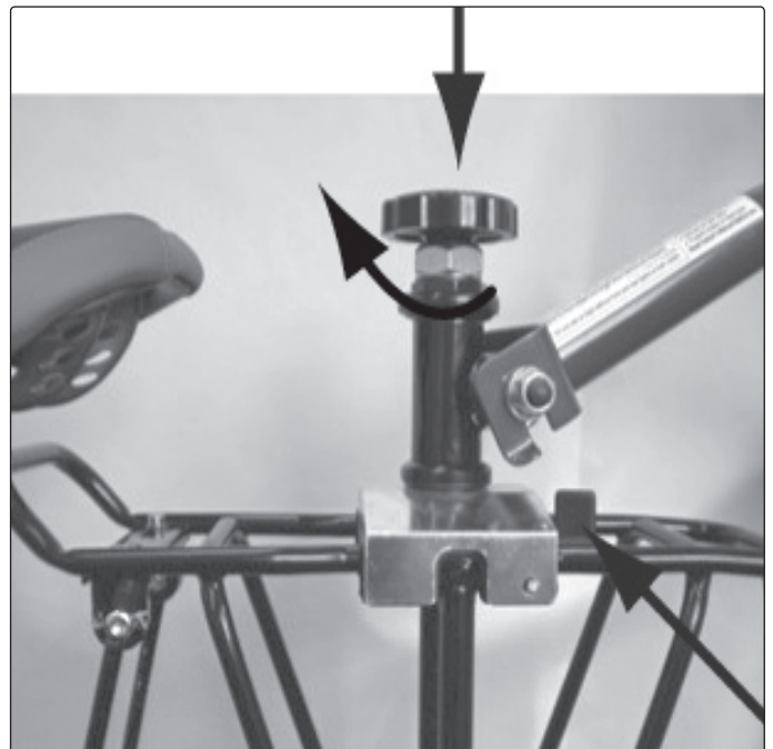
7 Trailercycle hitched to bike. Push down and turn to tighten as indicated by arrows.
