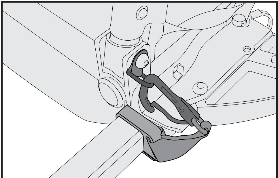
**ENG** The completed installation will look like this. The purpose of the red bracket is to provide a visual indicator that the tow bar has been inserted all the way, and the strap will keep the trailer attached to the bike in the event of an equipment failure.
