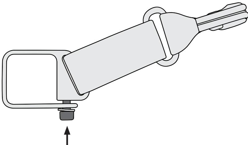
**ENG** 6. Tighten the screw on the bracket to lock it in place. Once installed on the tow bar, the safety strap is not to be removed! It will show you that the tow bar has been inserted all the way, and provide an extra layer of protection.
