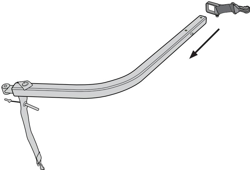
**ENG** 1. To install the safety strap, position the tow bar and safety strap bracket as shown. The orientation is important. The bracket bolt should be facing down, and the strap should be facing outward on the same side of the towbar as the detent.
