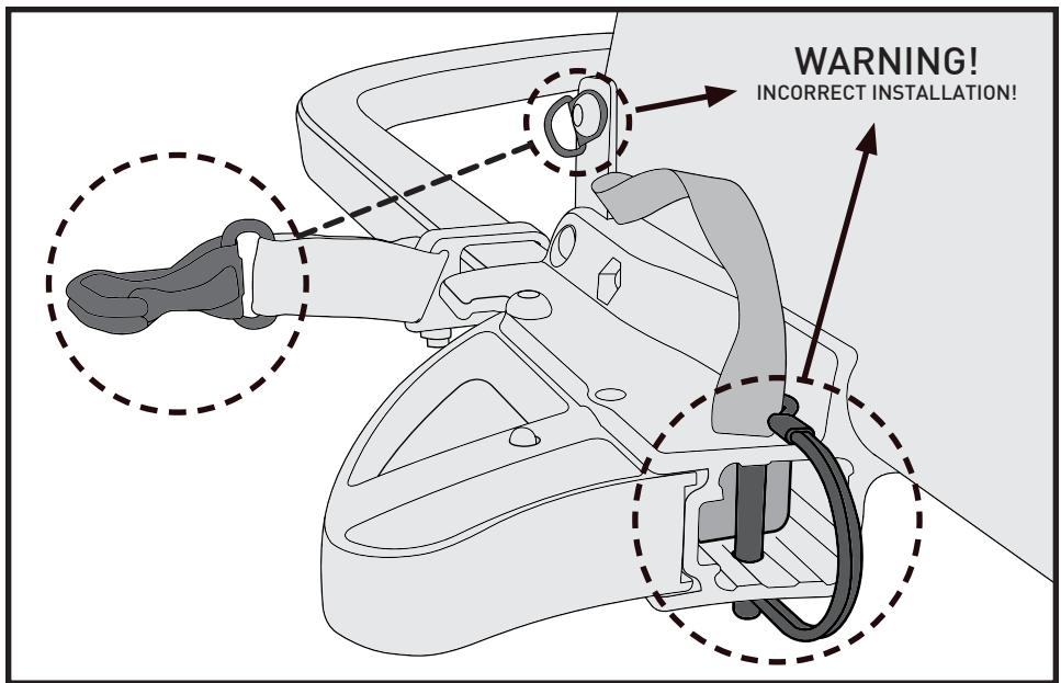
**WARNING!** This graphic shows an incorrect installation. The tow bar has not been inserted all the way, and the retaining pin is not going through it. Always make sure the retaining pin is going through the tow bar and receiver before it is locked. As shown in step 4. The safety strap must also be clipped to the D-ring.
