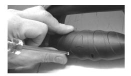
2. Cut the exposed section of the cable, then remove the white tubing and discard.
