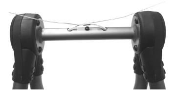
8. Make sure that the frame hinges are engaged (either in folded or unfolded position, but not in between.) Center the ferrule on the cross tube, then crimp the ferrule using crimpers or appropriate pliers. Make sure the ferrule is fully crimped, then trim the ends of the cables as shown. (The kit includes an extra ferrule in case you have difficulty crimping the first one.) Once crimping is complete, remove the tape holding the white tubing.
