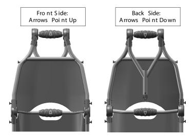
10. Capture the ferrule in the slot on the Twist Grip, then fasten the grips to each other using the four screws removed earlier, taking care to not strip the threads.
