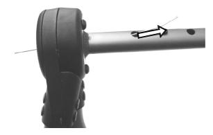
6. Slip the new white tubing over the free end of the cable and into the hole in the cross tube, leaving  $\frac{1}{2}$ " (13mm) of the tubing exposed. Tape the tubing in place temporarily to prevent it from slipping into the hole.
