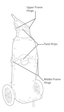
Your Travoy has two frame hinges: one to fold down the tow bar, and another to fold the frame in half. Both of these hinges are actuated by a cable at the twist grip. Should the cable release mechanism experience problems, this kit can be used to replace the cable mechanism.
