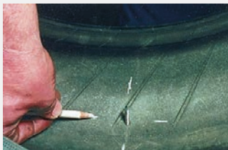
Remove the tyre and mark out the puncture on the inside
