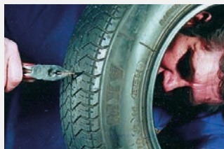
Pull the metal insert through the tyre smoothly and locate the plug patch
