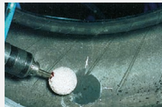
Lightly buff until curing bladder pattern disappears. Remove subsequent dust
