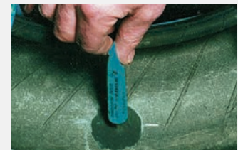
Apply vulcanising cement to the puncture area and into the hole. Allow 5 minutes to dry
