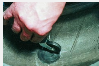
Roll down the patch from the centre outwards
