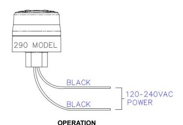
To operate the unit, just apply power. There are no adjustments to make for flash rate or intensity.
