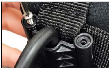
Step 5: Replace screws (2) on top side of entry point
