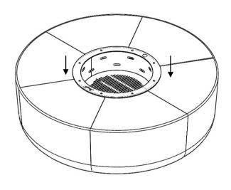
To assemble the benches join the two opposite parts and tighten them using the screws and nuts provided.
