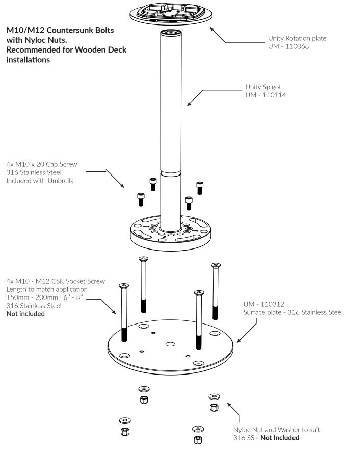
NB: It is the responsibility of the installer to ensure that any fixings used in the installation of the umbrella surface plate are suitable for the application
