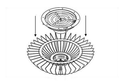
Install the glass with the help of the notches, so that it is fixed;
