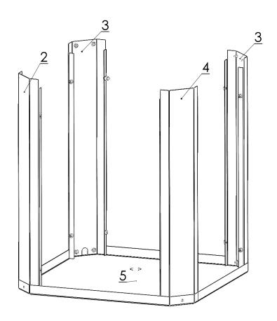
3. Mount bottom plate (No. 1) use 8 pieces M6 flange nuts to fasten the bottom plate to the corners. Make sure that the two small Ø5 holes for the door is pointing towards you.
