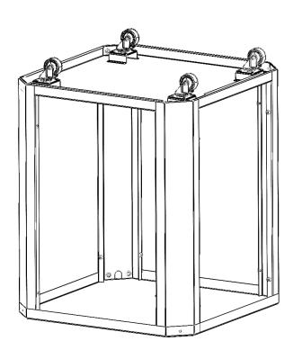
5. Turn the table around so it stands on the wheels. Mount the handle in the two holes in the top plate. Use 2 pieces M8x10 screws (packed together with the handle)
