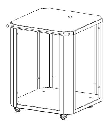
6. Mount the two side plates and the back plate. (All three plates are identically) Use 12 pieces M6x16 and 12 pieces M6 flange nuts.
