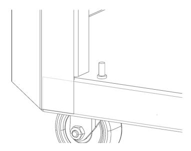
8. Mount the door on the pin in the bottom plate, push down the spring in the top and fix it in the hole in the top plate using your finger.
