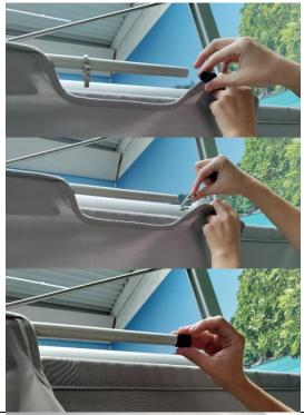
Unscrew the bolt on the head. For a spectra before 2022, it will be fixed in position 1, for the 2022 model, it will be in position 2.
