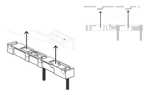
Note - before fixing bracket to the desk frame you will need to remove the screw at the rear of each frame side bracket (found in location marked by \*)
