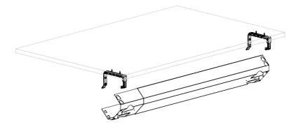
**EN** - Two different positions depending on height **A: 108 mm** or **B:140 mm** (NOTE! When mounting on a Classic Twin frame you can only use position A: 108 mm)
