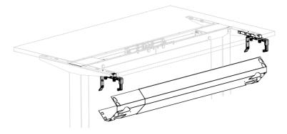
**EN** - Two different positions depending on height **A: 127 mm** or **B: 158 mm** (NOTE! When mounting on a Classic Twin frame you can only use position A: 127 mm)
