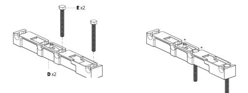
*Note - if fixing cable tray to a compact desk with 600mm depth desktop then insert hexagon bolts into the middle 2 holes of the bracket (marked by \*)*
