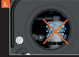
2. No water in the motor compartment. Contact support if you find water.
