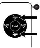
Simultaneously press and hold the HEAD UP and HEAD DOWN buttons on remote until the remote back lights blink, then release remote buttons.
