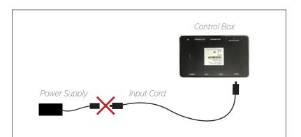
Connect the end of the Battery Backup Strap to the input power cord that is attached to the control box.
