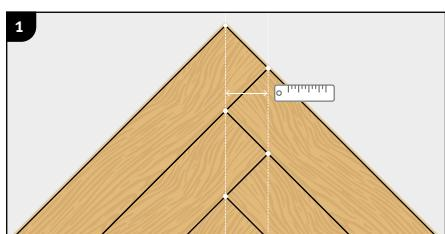
Measure the distance between the two straight lines, originating from the corners of the strips.
