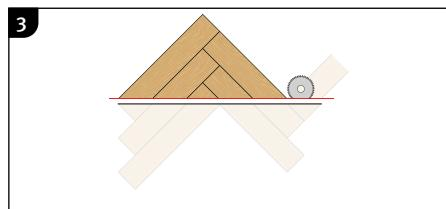
Cut the triangle according to the indicated red line. Depending on the kind of saw you use, it may be useful to dismantle the triangle before sawing.
