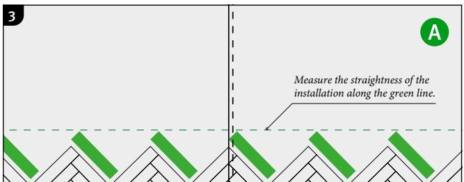
Install **A-strips** to connect all triangles. The joints between the A-strip and the triangle need to be checked very carefully. No protruding edge may be felt!
