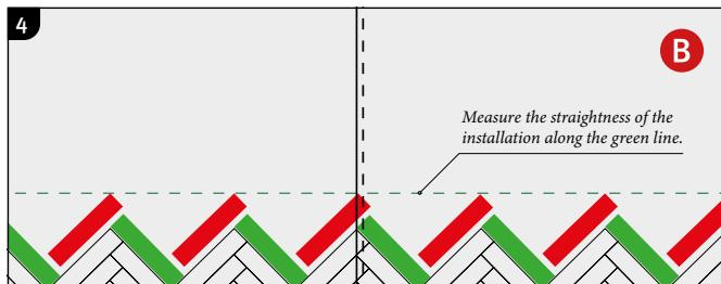
Now install **B- strips** and cut the most right piece to size.
