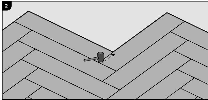
Use a rubber hammer and slightly knock at the 5Gi system to connect the short side. Start in the corner and work towards the end of the board.
