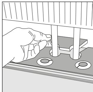
Drill holes two times larger than the diameter of the pipes. Remove a piece of the strip with a utility knife or a saw. Put the strip on one side of the pipes and the removed piece on the other side.
