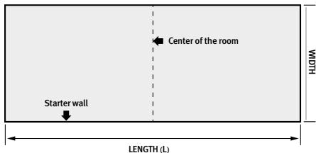
Define the wall from where you intend to start the installation. Mark out the center of the room.
