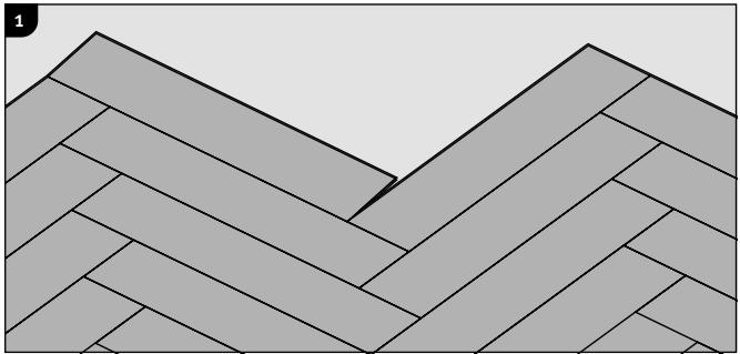
The boards need to be locked into one another, using the 5Gi system. To connect a new board you have to use a rubber hammer.
