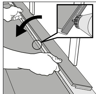
Remove the locking element according to the picture. Use applicable glue to connect the strips. Press- place wedges between the glued strip and the wall.
