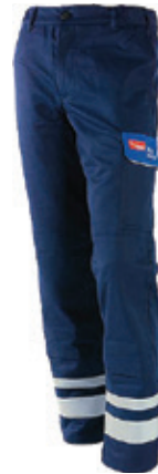
Arc Flash Trousers "Comfort", Class 1, HRC 2, 158 kJ, 13 cal / cm 2
