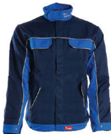
Arc Flash Jacket "Comfort", Class 2, HRC 2, 318 kJ, 22 cal / cm 2
