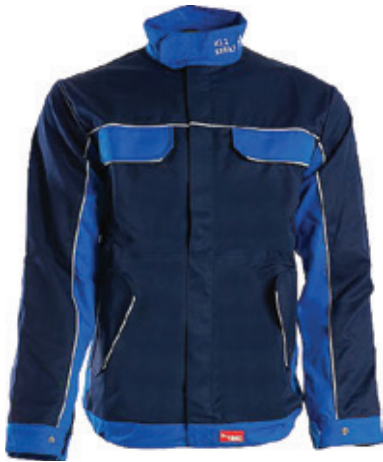
Arc Flash Jacket "Comfort", Class 1, HRC 2, 158 kJ, 13 cal / cm 2
