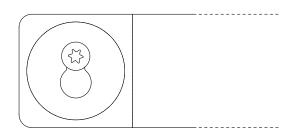
Place the large hole over the screw and gently push down the Wall Bar until it locks in place. Adjust the screw accordingly to make sure the bar seats securely in the slot.
