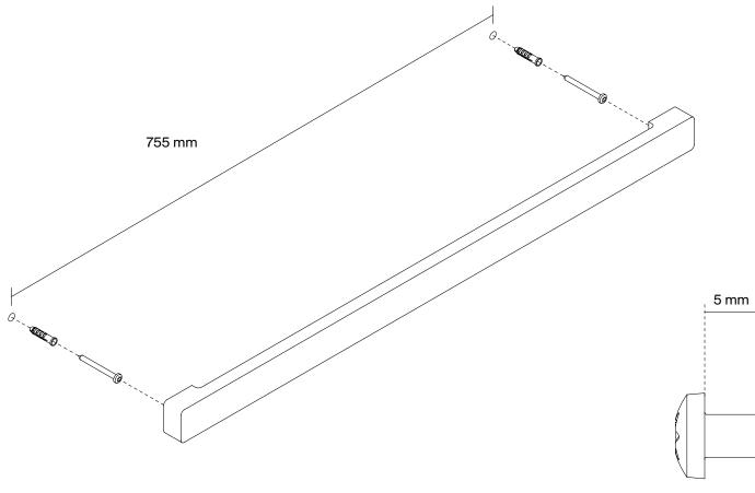
Mark two points, using a ruler and a spirit level. Distance 755 mm.
