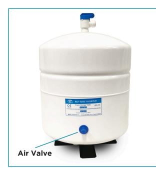
**NOTE:** The pre-charge on the Water Storage Tank is set at 7-10 psi by the manufacture. If the air pressure is low, remove the blue cap to expose the schrader valve. On an empty tank, add air using a standard floor pump.
