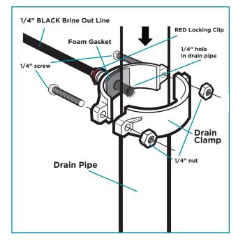
**NOTE:** To avoid drainage noise, mount drain line as low as possible on the vertical tailpiece, or on horizontal tailpiece.
