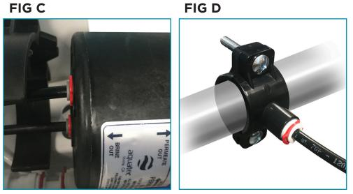
2. Connect the 1/4" **BLACK** tube from the Permeate Pump Brine Out **(C)** to the Drain Saddle Valve **(D)**.
