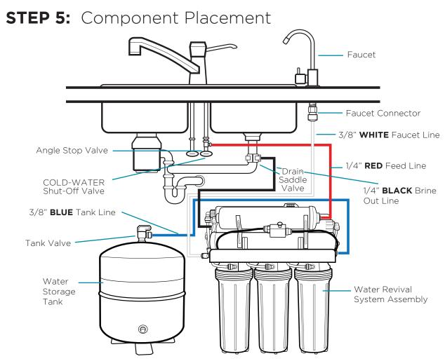
**LOCATION:** Though most often thought of as an under the kitchen sink counter device, locating the system in a basement, laundry room, or garage may also be convenient, depending on your circumstances.
