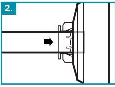
Tubing is secured in position.
