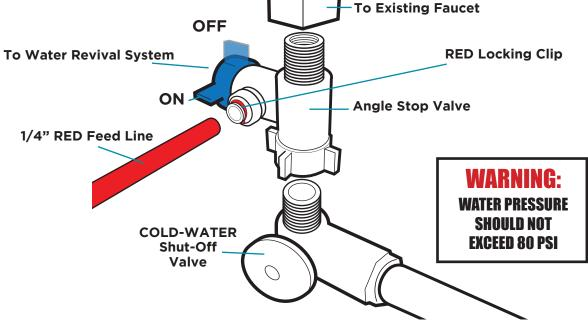
1. Locate the COLD-WATER Shut-Off Valve underneath the sink and turn it OFF.
