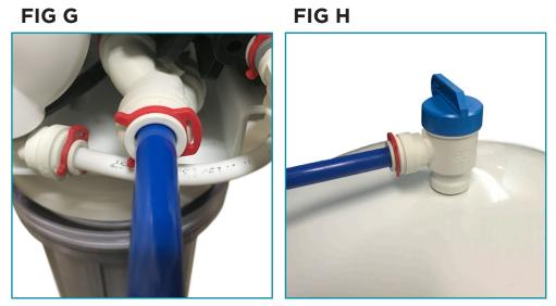
4. Connect the 3/8" **BLUE** tube to the RIGHT SYSTEM PORT **(G)** and the Tank Valve **(H)**.
