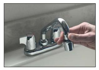
**1. REMOVE AERATOR** from the faucet you are trying to attach the system to. If it's too tight to remove by hand, use a wrench or pliers. If you have never removed the aerator before, you may find that it is very difficult to remove.
