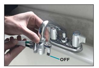
2. DIVERTER VALVE - Depending upon the thread type and depth of your existing faucet you may need to install one of the provided faucet adapters. Once determined, firmly tighten adapter in place of aerator (See pg. 8). Now you can fasten the diverter valve to the faucet. Be careful not to over tighten and do not use plumber's tape of any kind.
