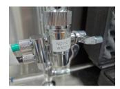
3. WATER PRODUCTION - Once the Diverter Valve is firmly in place, CLOSE the Valve by turning the lever to the horizontal position. If the valve is in the OPEN position, water will run freely out, bypassing the filters.
