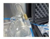
4. Now it is safe to run COLD-WATER through the system. OPEN the Fill Valve on the **BLUE** 1/4" tubing to dispense the product water. Waste water will exit through the **BLACK** 1/4" tubing and out of the Diverter Valve.
