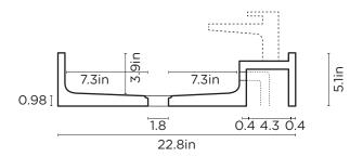
Note: Overflow pipe separate. For surface mount basin, a second hole in bench top is required.
