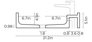
Note: Overflow pipe separate. For surface mount basin, a second hole in bench top is required.
