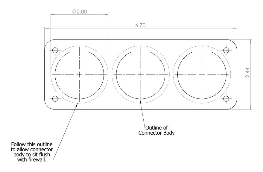
\*NOTE, THIS IS A SCALE DRAWING FOR THE MOUNTING PLATE. MAKE SURE WHEN PRINTING THAT YOU ARE USING STANDARD 8.5"X11" PRINTER PAPER AND SCALE IS SET TO 100%\*
