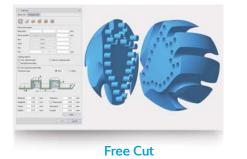
Cut with advanced cutting lines: define the cutting directions by 3 points plane, tangent plane, vertical plane, XY plane, XZ plane, YZ plane, polygon, circle, rectangle and section.
