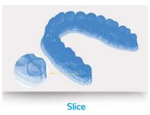
Slice parts with any layer size, and you can set different layer size in different area of parts for adaptive slicing, and visualize the contours of each slice conveniently.
