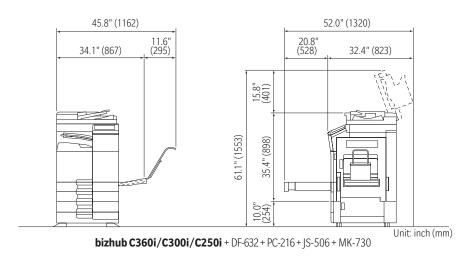
NOTICE: Be sure to allow a clearance of 8 inches (200 mm) or more at the back of this machine for the ventilation duct.
