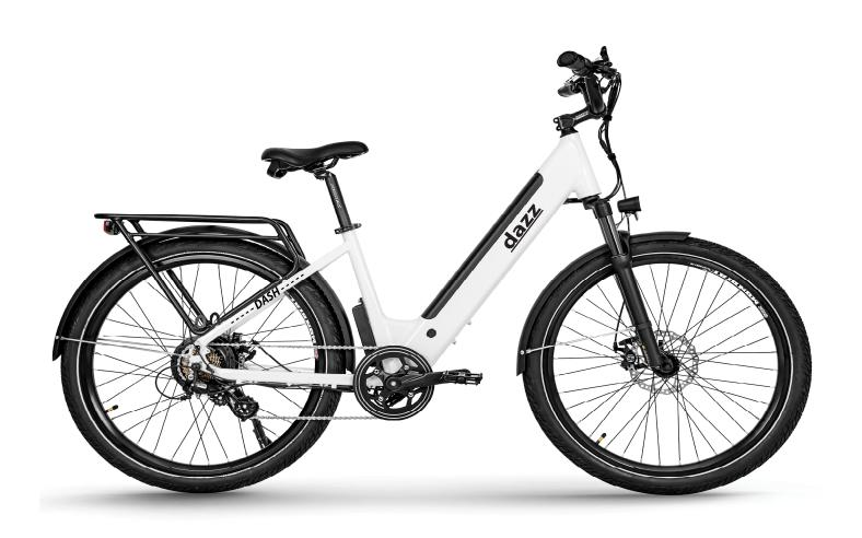
The 27.5" x 2.4" Panasonic puncture-resistant tires prevent punctures by sharp materials. A bit wider than ordinary tires makes the commuting journey smoother. Removable 48V 16AH Lithium-ion battery meet a 90km commuting journey. Continuous 500W brushless gear hub motor with a peak value of 750W makes crossing urban blocks and hills an ease. Fast and smart 48V 3 amp charger only takes 5 hours to fully charge the battery.
