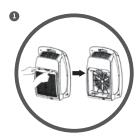
Simultaneously press the two buckles to open Back Cover.
