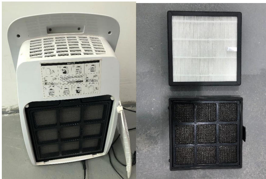
NCCO Filter and HEPA
