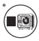
Place the Pet NCCO Reactor into the air purifier.
