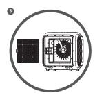
· Place the NCCO Reactor into the air purifier.
