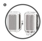
Unplug the appliance, find the two grooves under the front panel, and remove the front panel by pulling it outward.
