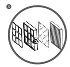
Install HEPA filter, static filter and pre-filter in sequence into HEPA filter frame.
