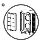
Place the HEPA filter and the pre-filter onto the NCCO reactor.
