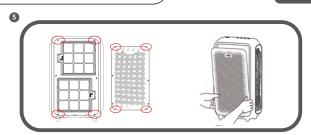
Align the front cover with the four positioning posts on the body, gently push inward, and the magnet will attach tightly to the body, and the front cover installation is complete.
