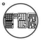
Install the upper NCCO Reactor and HEPA Filter Frame in sequence into the device. There is a click sound to indicate all the filters install successfully. Lower filters installation is as above.
