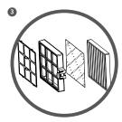
Install HEPA filter, static filter and pre-filter in sequence into HEPA filter frame.
