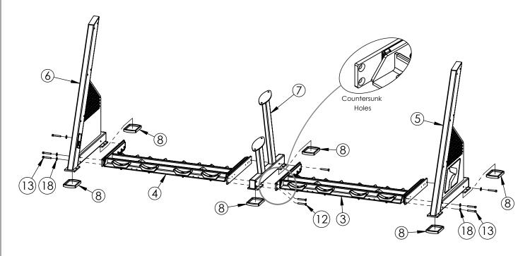
Step 1: Fit Rubber Footpads (7) onto the support frames as shown. Assemble the Right Drawer (3), Left Drawer (4), Right Support (5), Left Support (6), and Middle Support (7) together as shown, using the appropriate fasteners. Do not tighten any bolts until mentioned in Step 5.
