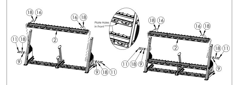
Step 2: Bolt one Middle Shelf (2) through the lower set of holes in the Right and Left Supports. Orient the Middle Shelf such that the holes for the numbered plates are in the front.
