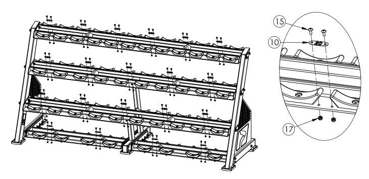
Step 6: Attach the numbered weight plates (10) to the shelves and drawers using 1/4" Screws (15) and Flange Nuts (17).
